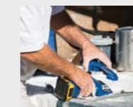
2) Remove the old pump from the sprayer
