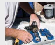
3) Place new pump into sprayer
